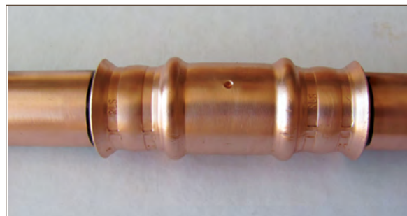
Figure 11.17. Completed joint showing double 360° crimps
