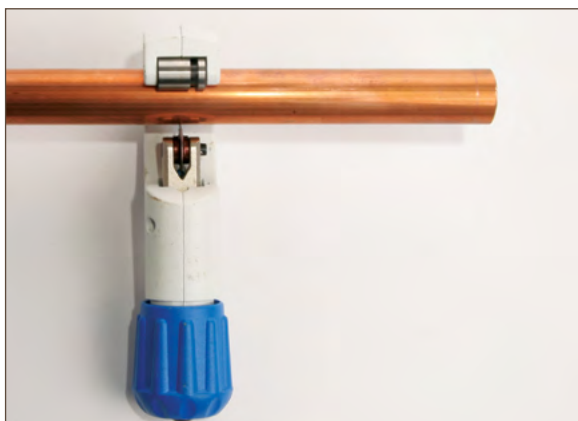
Figure 11.6. Cutting the tube square
