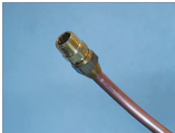
Figure 9.2. Completed Flared Joint
