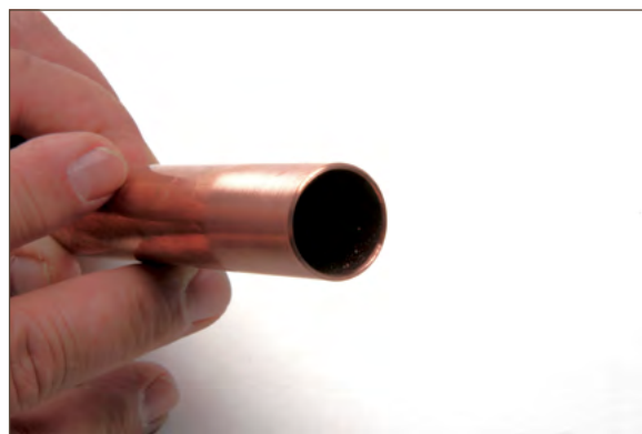
Figure 13.8. Reamed and deburred branch tube end
