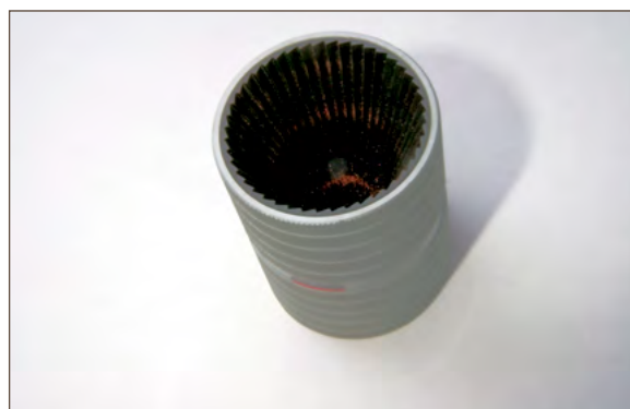
Figure 11.9. Combination tool for I.D. and burr removal
